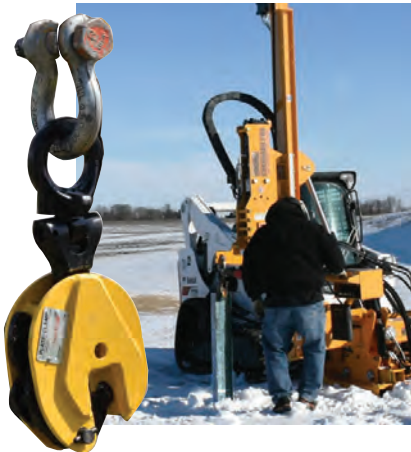
Pile Puller Kit features a 1 ton vertical lift plate clamp and safety shackle attached to the steel pull plate on the front of the mast and hammer. The vibratory assist, and a vertical pull capacity of 2000 lbs (1 ton) removes pile/post from the ground. This accessory can easily be removed when not in use or while transporting. Part No. 360267
