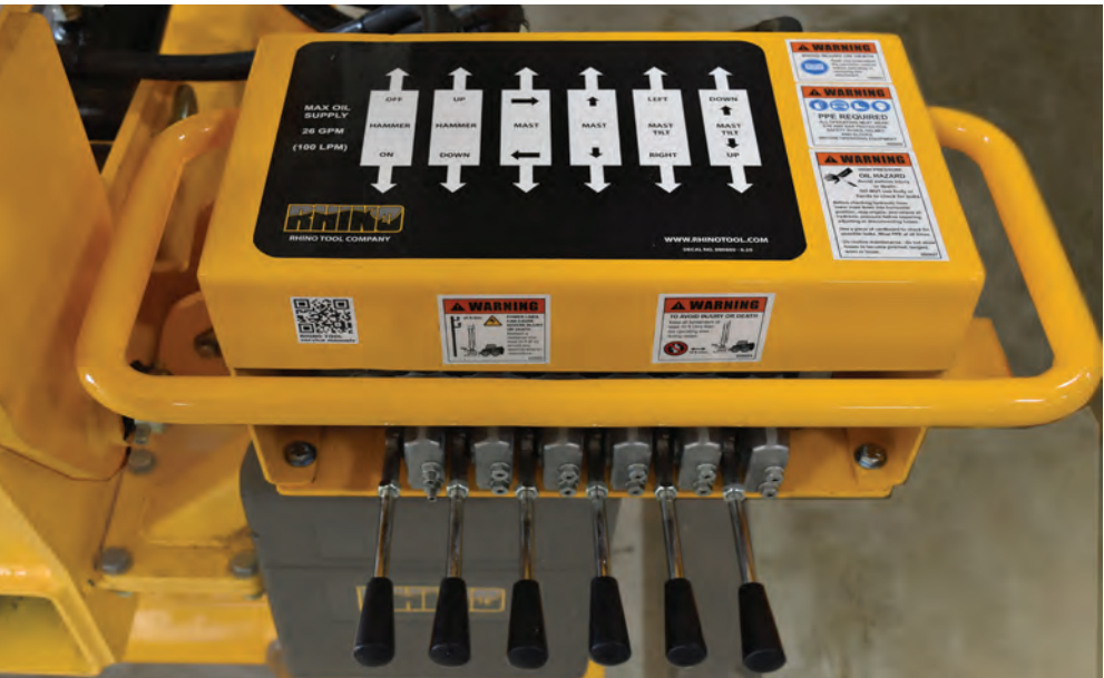
Omni Directional Adjustment for precise positioning and leveling of the pile and to accommodate for Uneven Terrain
