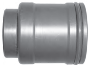
Fig. 14 - Small end of Hammer is toward the anvil.
