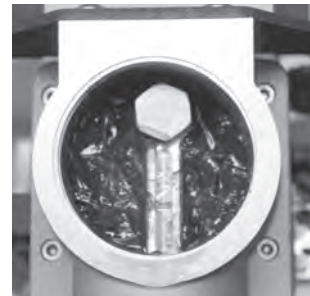
Fig. 11 - After completely cleaning out old Lubricant, add new Rhino® Pro Series Lubricant till level with the bottom edge of the crank pin head.
