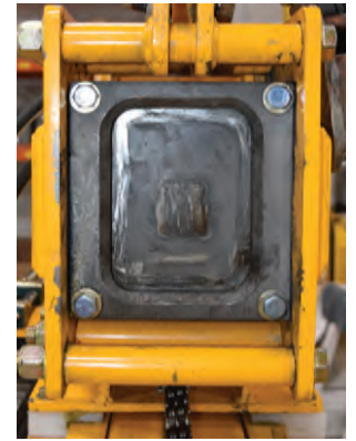
Removable adapter plate, shown above. Custom sizes and shapes available.
