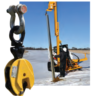
Pile Puller Kit features a 1 ton vertical lift plate clamp and safety shackle attached to the steel pull plate on the front of the mast and hammer. A vertical pull capacity of 2000 lbs (1 ton) removes most pile/posts from the ground. This accessory can easily be removed when not in use or while transporting. Part No. 360267
