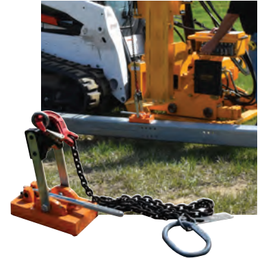
Pile Lift Kit features a magnetic lift assist that attaches to the pile or post. With a rated lift strength of 1378 lbs and a max pull-off strength of 550 lbs, this accessory aids the operator in manipulating the pile/post from the ground into a vertical position. This accessory can easily be removed when not in use or while transporting. Part No.360270
