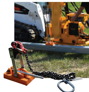
Pile Lift Kit features a magnetic lift assist that attaches to the pile or post. With a rated lift strength of 1378 lbs and a max pull-off strength of 550 lbs, this accessory aids the operator in manipulating the pile/post from the ground into a vertical position. This accessory can easily be removed when not in use or while transporting. Part No.360270
