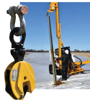
Pile Puller Kit features a 1 ton vertical lift plate clamp and safety shackle attached to the steel pull plate on the front of the mast and hammer. A vertical pull capacity of 2000 lbs (1 ton) removes most pile/posts from the ground. This accessory can easily be removed when not in use or while transporting. Part No. 360267
