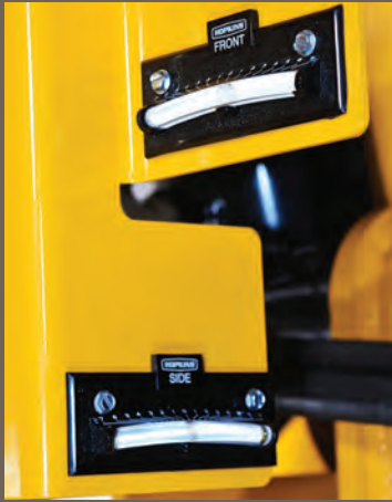
Two quick-read, numbered, leveling indicators to plumb pilings.
