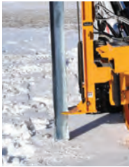
Bottom Guide secures Pile - Custom sizes and shapes available.
