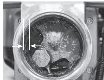
Fig. 10 - If ridge of Rhino® Pro Series Lubricant measures 1/8" or less, add a small amount. At maximum level it should measure 1/4".
