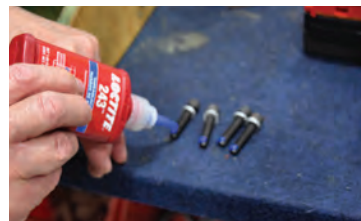
Fig. 18 - Use Loctite 243 (blue) on all bolt holes and bolts
