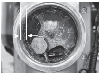
Fig. 10 - If ridge of Rhino® Pro Series Lubricant measures 1/8" or less, add a small amount. At maximum level it should measure 1/4".
