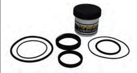
Ranch Pro Service Kit Part No. 300508: (# location indicated on exploded parts diagram) (#8) O-Ring Seal for Piston and Hammer - P/N: 300600 (Qty. 2) (#26) O-Ring Seal for Pro-Series Crankcase Cover - P/N: 301617 (#12) Large Retainer O-Ring Seal - P/N: 300604 (Qty. 2)
