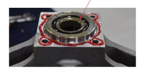
Fig. 12 - Proper preparation of the Lower Body retainers, o-rings and Loctite 518 (red) before re-attaching to the Upper Body Assembly
