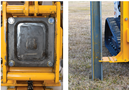
Adapter Plate & Bottom Foot, secures a 4.5" x 6" Pile - Custom sizes and shapes available.
