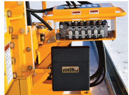
Control center, Operation Manuals and Solar Pro specific tools centrally located for operator.
