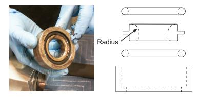
If the elements in the anvil o-ring cup need to be reassembled, do so in this order: 1.) lower o-ring; 2.) large retainer with radius to the top; 3.) top o-ring. Then insert assembled anvil o-ring cup into the lower body.
