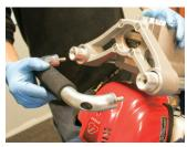
the throttle into a center position and tighten the hex nuts with a 5/32" (4mm) hex key. Set out the top handle bolts and apply Loctite 7649 Primer N to threads of each bolt and to bolt holes on the handles followed by an application of Loctite 243 thread locker to bolt holes on top of side handles. Using acetone or solvent, clean and springs and inside of handle collars, then apply grease to both.
