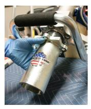
Place lock washers (300750-4), over the chuck bolts (300717-4) and apply Loctite 7649 Primer N to threads of each chuck bolt and to chuck bolt holes on the lower body and allow them to dry. When dry, apply Loctite 243 thread locker to threads of bolt holes.
