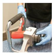
Position the handle and lower body as shown and with a soft mallet carefully strike the bottom of the anvil to dislodge it, then grasp it with your hand and slide it out. Set it aside and store in a convenient place for future use.
