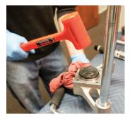
Stand the handles and lower body in the upright position. Insert the lubed anvil with o-ring into the lower body. If it does not seat completely, tap it lightly with a soft mallet to seat in proper position. It may be a tight fit.
