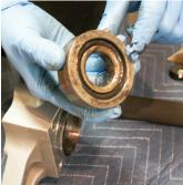
Remove the entire anvil o-ring cup with contents intact from the lower body.
