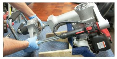
Set out the lower body bolts (300702-4 or 300701-4) and apply Loctite 7649 N Primer to threads of each bolt and to bolt holes on the upper body and allow them to dry. When it has dried apply Loctite 243 thread locker to bolt holes on the bottom of the upper driver body.
