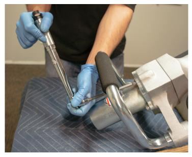
Finish the installation by using a torque wrench equipped with a 1/4" hex bit. Set the torque wrench to 251 in/pounds and torque the bolts in the same crossing pattern.
