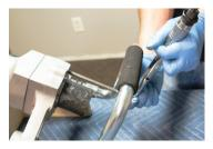
Insert and thread by hand the lower body bolts (300702-4 or 300701-4). Tighten them into place with a 1/4" hex bit socket in a crossing pattern, then with a torque wrench set to 251 in/ lbs torque the accordingly in the same crossing pattern. Slide
