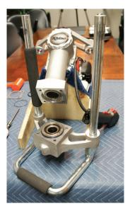
Separate the lower body from the upper driver body and slide the throttle off the end of the handle. Remove the gasket and sleeve o-ring from the lower body and
