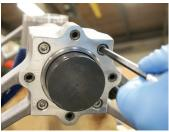
Remove the four lower body bolts at the bottom of the driver with a 1/4" hex bit socket. Clean any dried threadlocker from the bolts and the bolt holes to ensure all debris from previous installation has been removed.
