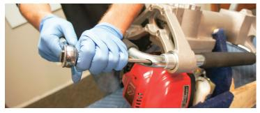
With a 1/4" hex bit tighten the 2 bolts into the handle. With a torque wrench set to 132 in/pounds (15Nm) torque the bolts.
