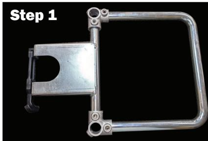
Slide "B and C", from Step 1, over "A" as shown. Position to best height for your post driver, and then tighten (2) "BB" with 1/4" Hex Wrench.
