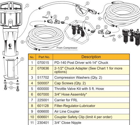
\*Made to order at desired length - additional charge per foot of hose
