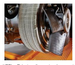
The HPP's efficient cooling system keeps out dirt and debris. Easy access allows cleaning of the radiator with a low pressure washer. (Less than 500 psi.)
