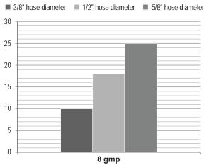
Pressure from Power Pack: 2175 psi (150 bar) Flow: 8 gpm,(30 lpm) zero elevation 2 set couplings per 32.8' hose
