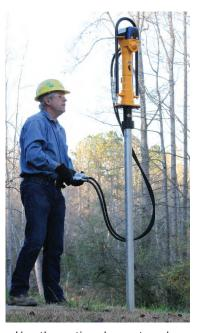
Use the optional remote valve (801011) with the HPD 60 tor driving tall posts.
