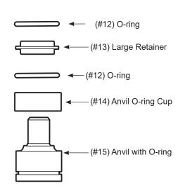
Insert O-ring into Anvil O-ring Cup, then insert Large Retainer (with large radius at bottom towards the anvil), then insert other O-ring.
